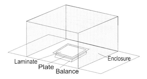
Figure 17.1. Typical Balance Enclosure
