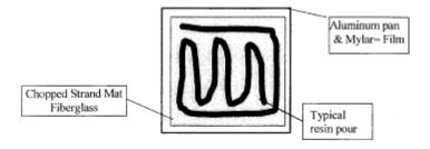
Figure 11.6 Resin Distribution Diagram
