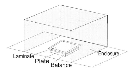
Figure 17.1. Typical Balance Enclosure
