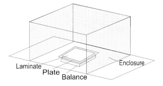
Figure 17.1. Typical Balance Enclosure
