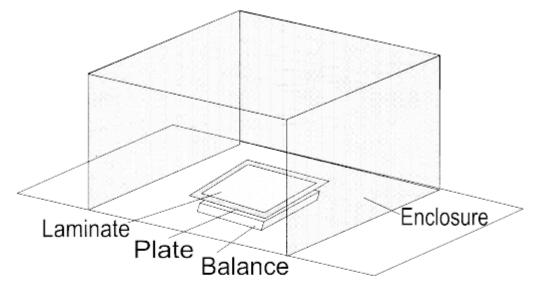
Figure 17.1. Typical Balance Enclosure
