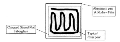
Figure 11.6 Resin Distribution Diagram
