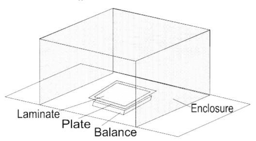
Figure 17.1. Typical Balance Enclosure
