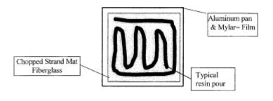
Figure 11.6 Resin Distribution Diagram
