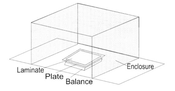
Figure 17.1. Typical Balance Enclosure
