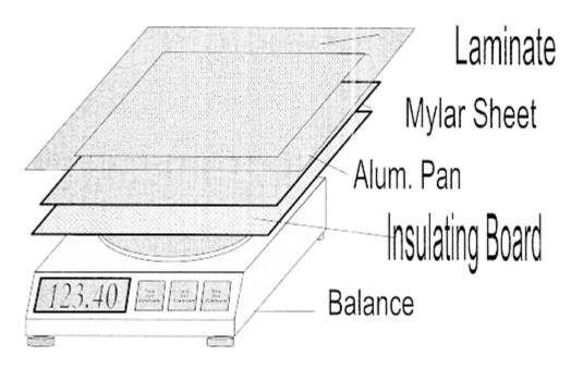
Figure 17.2. Scale, Plate, Insulating Board, Mylar, Laminate Order
