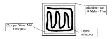
Figure 11.6 Resin Distribution Diagram
