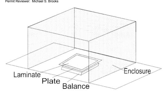
Figure 17.1. Typical Balance Enclosure
