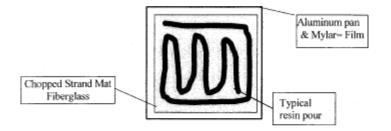
Figure 11.6 Resin Distribution Diagram
