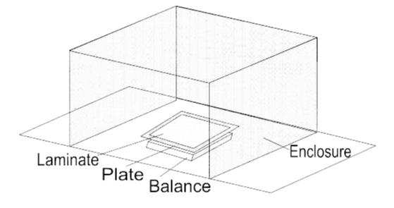
Figure 17.1. Typical Balance Enclosure
