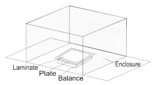
Figure 17.1. Typical Balance Enclosure
