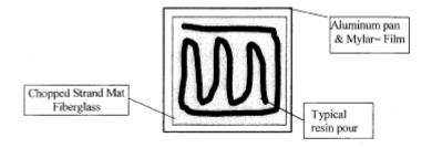
Figure 11.6 Resin Distribution Diagram
