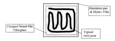
Figure 11.6 Resin Distribution Diagram
