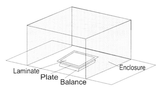
Figure 17.1. Typical Balance Enclosure
