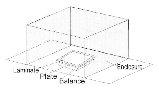
Figure 17.1. Typical Balance Enclosure
